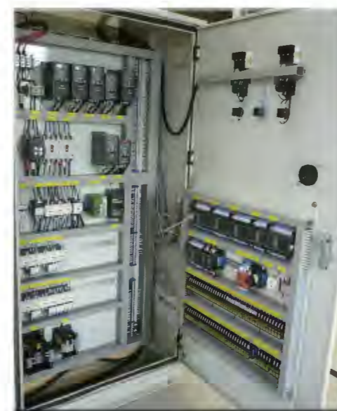
▲ All operation functions are controlled through a programmable logic controller. The machine has been passed CE safety measure identification. 電控系統經由PLC程式控制器控制系統，穩定檢修容易。歐規CE安全認證通過，安全性優越。
